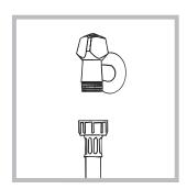
1. Connect the inlet hose by screwing it to a cold water tab using a 3/4 gas threaded connection (see figure). Before performing the connection, allow the water to run freely until it is perfectly clear.
